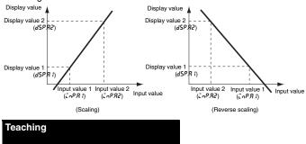
Settings for scaling can be made using the present measurement values instead of inputting values with the SHIFT and UP Keys. This is a convenient function for making the settings while monitoring the operating status.
