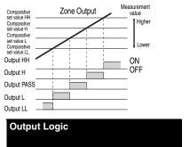
Reverses the output operation of comparative outputs for comparative results.
